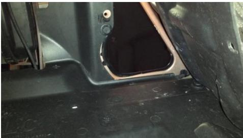
Install supplied edging material (this step will be the most frustrating step and requires a little heat to soften the material and activate the adhesive inside the material. a little patience goes a long way!)
