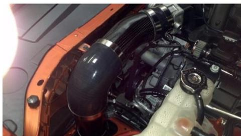
Carefully install IAT sensor into grommet hole in lower tube. (the use of a little lubricant will aid in the insertion of the sensor)
