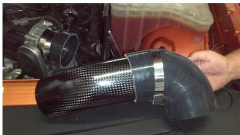
Install as one piece and check alignment of tube. You want top tube to be square and parallel.
