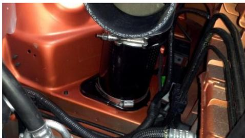
Install 3.5"-4" reducing coupler onto throttle body and assemble the upper tube to the 90\* silicon elbow. (all clamps are in place loosely!!!)
