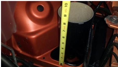
Install 4" worm clamp as seen in picture. This is to secure the lower tube from migrating down. This may be adjusted at the final point of install to get the intake level.
