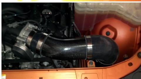
Position all clamps so bolts are to the underside of the tubes. This looks cleaner and acts a point to secure the IAT extension harness in the next steps.
