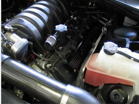
For later Gen II & III cars (2011 - present) install by trimming off a 1.5" peice of the OEM breather tube and using it as a "coupler" to attach the breather filter in a similar manner as shown below. You will have to remove the small worm clamp on the breather filters when connecting in this manner.
