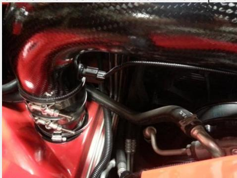
Finally, install the breather filter to the fitting coming off the oil fill neck. There are multiple ways to do this and you can use your creativity. I recommend with early Gen I cars (2005 - 2010) to install the breather directly onto the filler neck fitting
