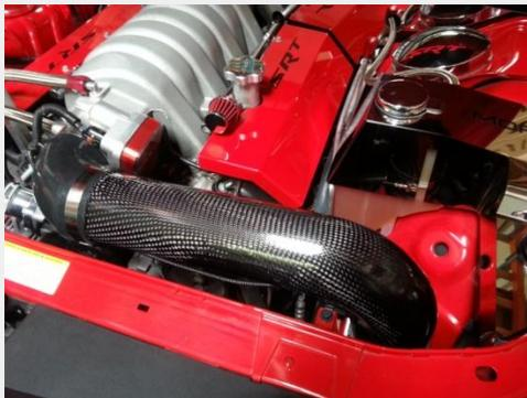
Make necessary adjustments with the tubes in order to get the upper tube to sit level with the radiator support and tighten clamps. The 4" worm clamp used initially to hold the lower tube in place will continue to be utilized as a means to level the upper tube and to keep the lower tube from migrating downward **DO NOT OVER TIGHTEN THE CLAMPS ON THE CF TUBES. THINK "SNUG". OVER TIGHTENING CLAMPS CAN RESULT IN DEFORMATION OF TUBES OVER TIME.**
