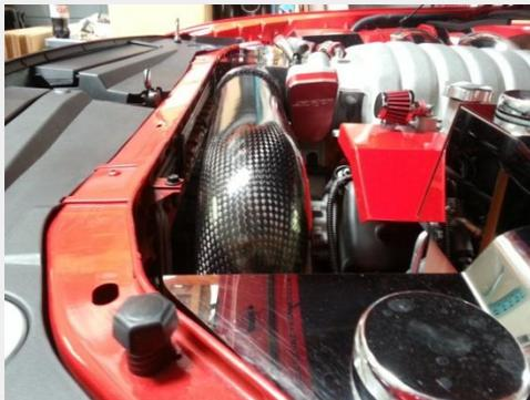
Next install IAT sensor into grommet as shown below and install the IAT extension harness that is supplied in the kit. Use the supplied black zip ties to secure the IAT extension harness to the clamp at the throttle body and the other zip tie will go through the plastic ring attached to the underside of the tube. (note the placement of the 4" worm clamp. This is the manner described in the previous step)
