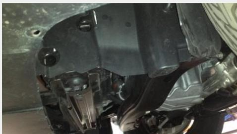
Note: It can be advantageous for some to remove the driver's side wheel and pull back the inner plastic fender liner to gain even better access to the area where the filter will reside on the initial install. The view would be as seen below
