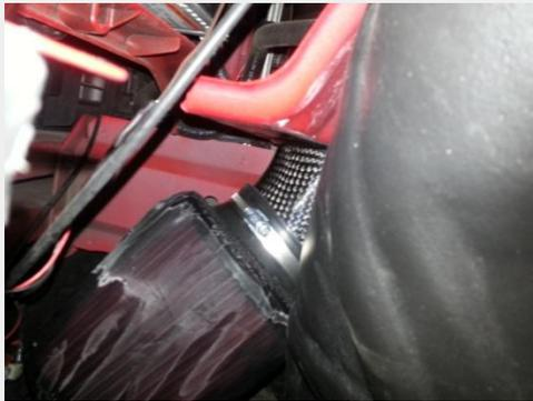
Once the tube is installed, put the 4" worm clamp supplied around the tube to temporarily hold it in place. You can also install the supplied 4" straight silicon coupler at this time.
