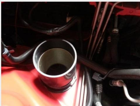
Next, install (2) of the (3) 4" T-bolt clamps that are supplied in the kit, around the silicon coupler. Leave clamps loose at this time for later adjustments.
