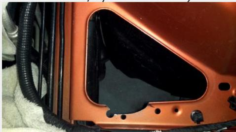
Be sure to notch the lower plastic baffle that is attached just under the area to be notched. It is held in place with standard fenderwell push pins.
