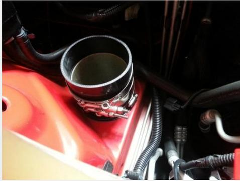
Next, install the 90\* 3.5" - 4" silicon elbow onto the throttlebody. Leave clamps loose for later adjustments.
