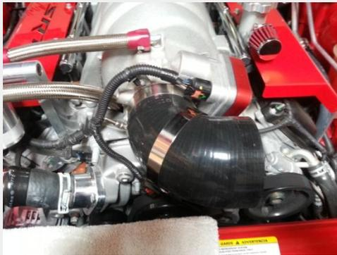
Next, install top 90\* carbon tube to connect the silicon elbow and the down tube previously installed.
